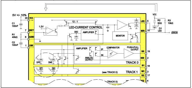
Fig. 1: LED Current Control and Monitoring
