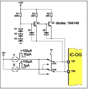
Fig. 2: Wiring the test aid
